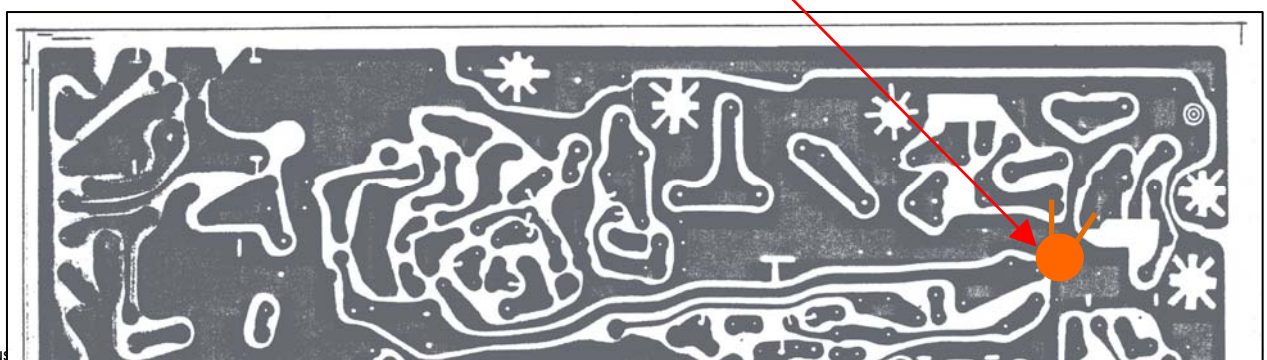
30pF – 68pF capacitor in parallel with C62
